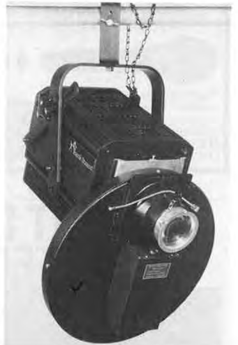
Cadenza EP 2000W Effects Projector fitted with Moving Effects Attachment and Objective Lens.
